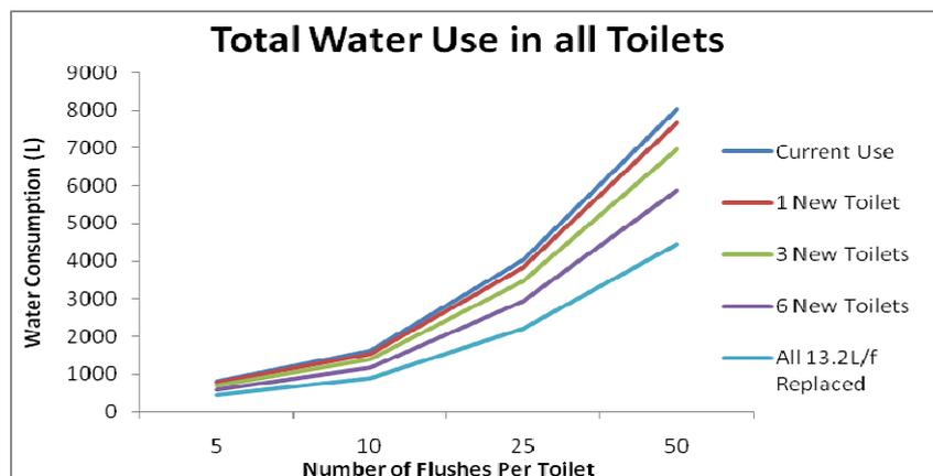
Figure 6: Arena toilet water use values are shown by number of flushes. "Current Use" is the amount used with all ten 13.2 L/f toilets, every subsequent line being the new usage if the specified number of these high flow toilets were replaced with 6L/f toilets.
