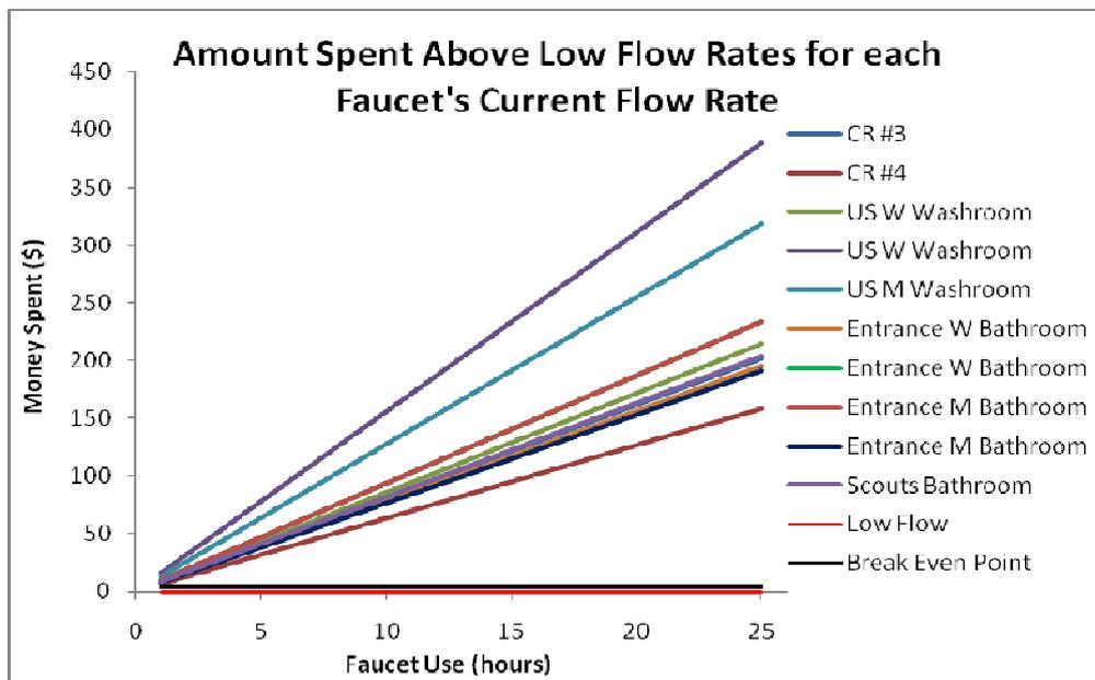
Figure 2: The arena faucet flow rates were analyzed by the extra amount of money spent when using the current fixture instead of a low flow faucet (low flow = 6L/min). The low flow line is on the x-axis because this chart displays the amount of money spent on the flow which exceeds this low flow rate, and the breakeven point (\$4.00) is where the black line meets the shower lines. In these charts, CR always stands for change room, W is for women's, M for men's and US stands for upstairs.
