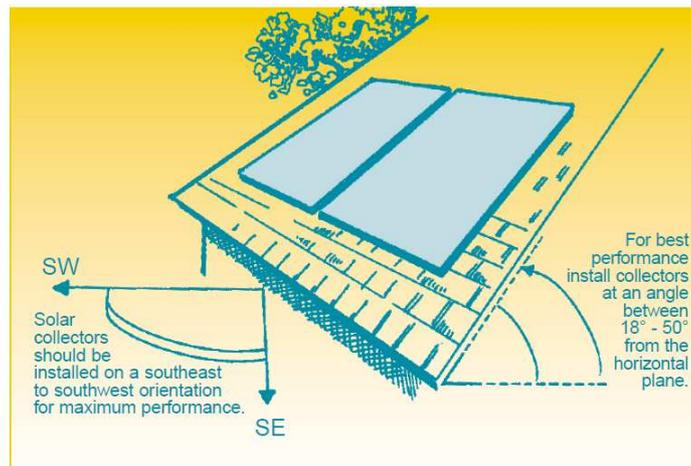
Figure 9: Diagram showing the optimal placement of solar collectors (Natural Resources Canada, 2000).
