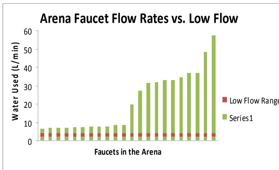
Figure 1: Arena faucet flow rates measured in L/min. The average range of low flow faucets are shown in red.
