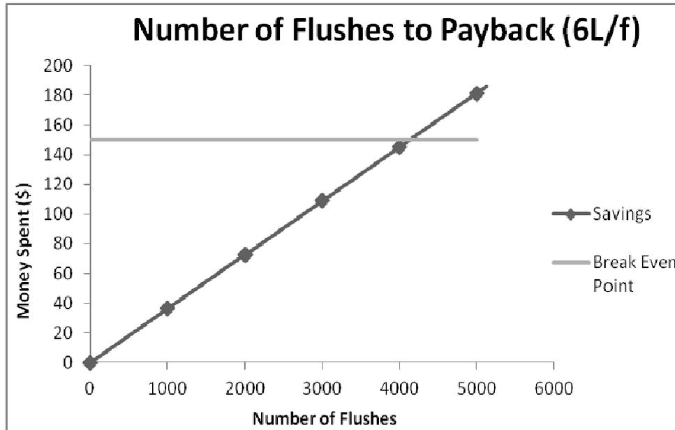
Figure 7: The payback period for replacing a 13.2L/f toilet with a 6L/f toilet priced at \$150 is displayed. The increasing line shows the money saved over the number of 6L flushes (saving 7.2L a flush). The breakeven point is where the two lines meet, anything above that is savings.
