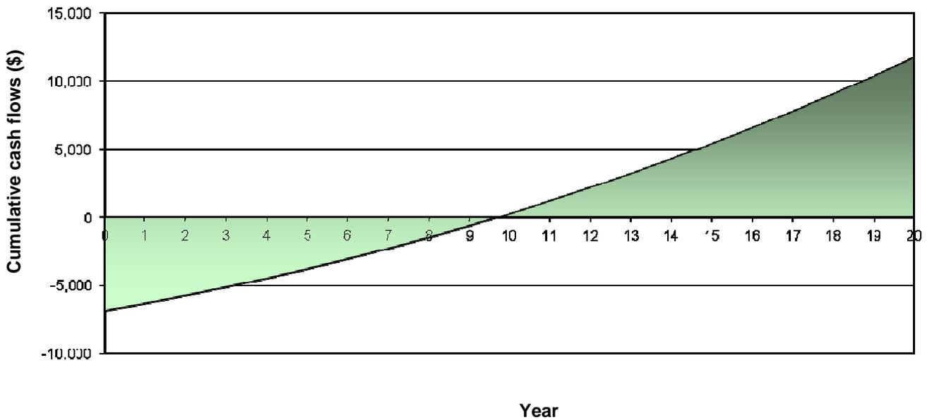
Figure 10 : Payback period on the solar hot water system for the dishwasher, showers and faucets is displayed. The point in which the line reaches the x-axis is the breakeven point for the project, and everything above the x-axis is money saved.
