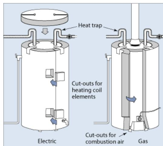
Figure12: Diagram showing insulation of electric and gas water heaters (DOE, 2011).
