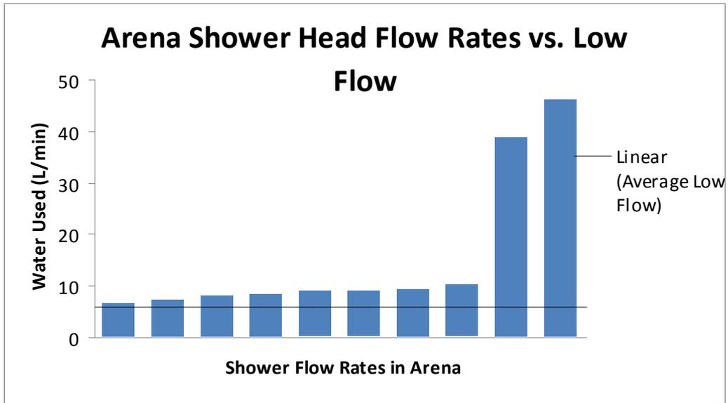
Figure 4: Arena shower head flow rates measured in L/min. The average flow rate of low flow shower fixtures is shown as a black line.
