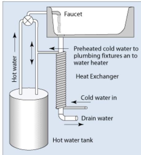
Figure 11: Diagram of a grey water heat recovery system (DOE, 2011).
